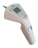
FREQUENCY RANGE: from 40 Hz to 110 MHzOPTIONS: calibration Jig (CCM JIG)FOR MORE INFORMATION: datasheet, manual, video
