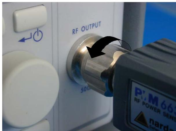
Disconnect the Fisher connector and the Data-Supply cable from the Power Sensor.
