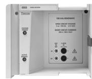
Plug-in module to produce the ring waves specified by ANSI/IEEE C62.41 Cat. A and B, and various UL standards, including UL 864
