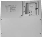
Module to produce the 10/250 $\mu$ s surges required by Telcordia GR-1089-CORE
