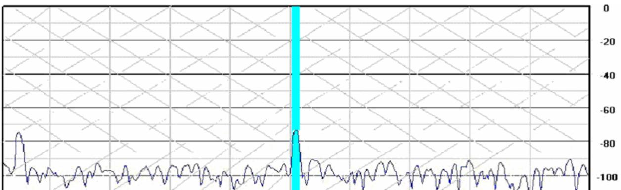
But the picture could be even worse as for the following picture where the signal is lower and the user can be misled thinking the signal is a spur, as many others present, and taking noise instead. As shown here below the error would result in an overestimation of about 10dB. Moreover, there might have been a thermal drift in the meantime (see
