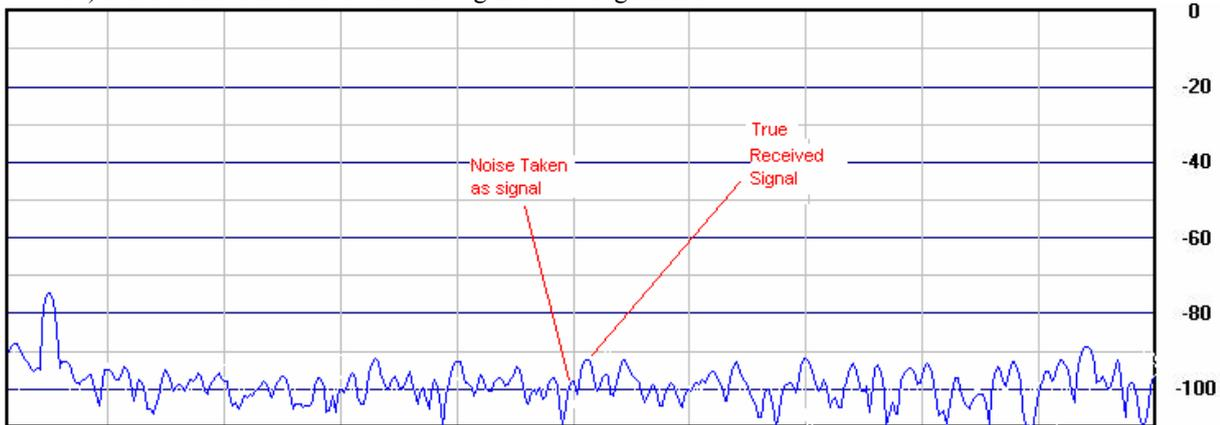
As a consequence, not only does not a spectrum analyzer add any useful information but it can even adversely affect the measurement as the user might be distracted from the real signal or, even worse, misled. And this comes very true when the user is not RF experienced.
