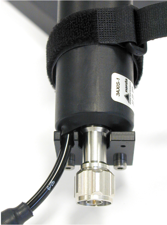
Figure 6: Cable and N connector in guideway
