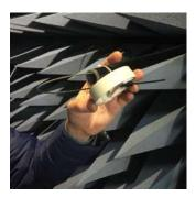
Anchor the sensor to the outreach, connecting the fiber optic
