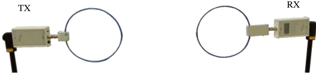
Picture 83 Example of coplanar orientation with horizontal polarisation
